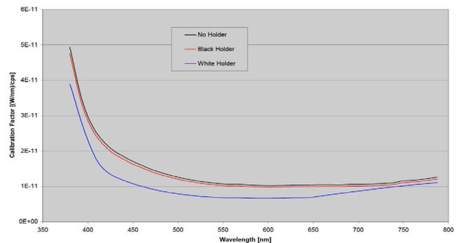
Figure 4. Calibrations of the OL 770-LED and OL IS-670-LED sphere with various LED holders.
