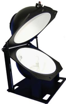
The horizontally-mounted seam of the OL 1800H 18" Integrating Sphere (w/ vertical opening) allows for an optional port to be placed on top of the hemisphere for testing downlights.
