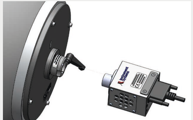
Figure 10: Use of an ACS 570 on an integrating sphere (luminous flux measurement)
